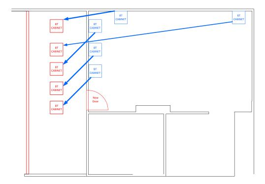
This would consist of BT disconnecting, moving, extending and reconnecting their existing cabinet and associated equipment. Initial estimates of time would be approximately 3 – 4 weeks, with significant down time for parts of the system but this will need to be investigated further with BT as part of stage 2 study.
