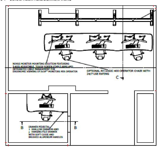
The control room will be stripped of all old equipment and furniture, one workstation will be paced is safe storage for the duration of the works. Please note, none of the current wall monitors will be re-useable for these works, four new monitors will be required for the new layout.
